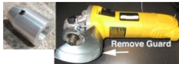
Figure 3. Convert an angle grinder into a high-speed drill with this specialized adaptor. It fits on a 5/8-11 spindle. This adaptor works only with high-speed drill bits.
